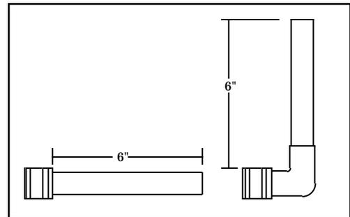
7. After soldering is complete, cool the pipe and connectors. Slide the plastic nuts (#1) over the brass connectors (#4). Place the white plastic split rings (#2) into the grooves closest to the copper pipe. Next place the O-Rings (#3) into the grooves closest to the end of the brass connectors (#4). Re-assemble the completed connection kit onto the bypass assembly. (see General Warning #8 on page 4)
