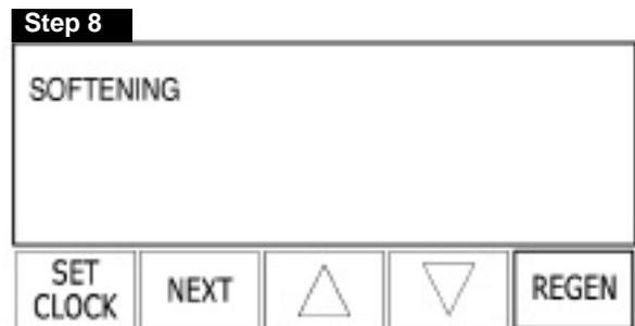
Once the drive motor stops, the manual regeneration is complete and the display will return to the normal display.
