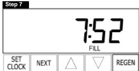
Leave the controller in this cycle until the float valve, located inside the salt container, shuts off.
