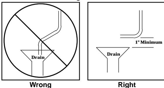
14. **Connecting the overflow line:** The brine overflow fitting is located on the outside of the salt container approximately 12" down from the top. Connect 1/2" drain tubing to the overflow fitting and run it to the nearest floor drain. This line is a gravity flow line and cannot be run overhead or cannot connect to a drain that is higher than the overflow fitting.
