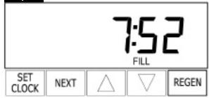
Leave the controller in this cycle until the float valve, located inside the salt container, shuts off.
