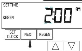
**STEP 4I** – Next Regeneration Time (hour): Set the hour of day for regeneration using ▼ or ▲ buttons. AM/PM toggles after 12. The default time is 2:00 AM. This display will show “on 0” if “on 0” is selected in Set Regeneration Time Option in OEM Softener System Setup or OEM Filter System Setup. Press NEXT to go to step 5I. Press REGEN to return to previous step.
