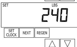
**NOTE:** Estimate the pounds of salt in the brine tank and add it to the amount of salt added to the brine tank. The example at the left would indicate 200 lbs. of salt being added to a brine tank that has 40 lbs. remaining.
