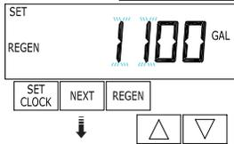
**Step 8S** – Set Volume Capacity using the ▼ or ▲ button. If value is set to:
