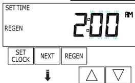
**STEP 5I** – Next Regeneration Time (minutes): Set the minutes of day for regeneration using ▼ or ▲ buttons. This display will not be shown if “on 0” is selected in Set Regeneration Time Option in OEM Softener System Setup or OEM Filter System Setup. Press NEXT to exit Installer Display Settings. Press REGEN to return to previous step.
