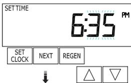
**STEP 3U** - Current Time (minutes): Set the minutes of the day using ▼ or ▲ buttons. Press NEXT to exit Set Clock. Press REGEN to return to previous step.
