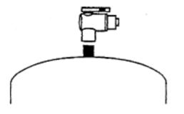
Note: Do not tamper with the air valve on the storage tank. It has been preset and screwed on with blue cap by the manufacuturers.
